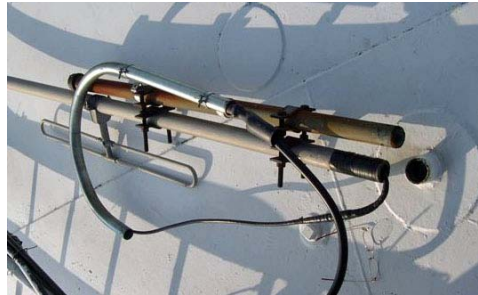
The CCARC's main repeater antenna broke away from its base following high winds.
